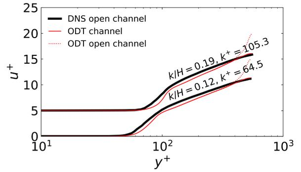
Figure 4. Mean velocity profiles.
