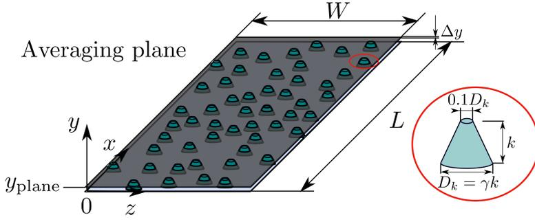
Figure 1. RAV and representative roughness element.
