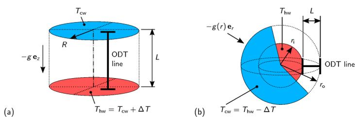
Figure 1: Schematic showing a planar (a) and spherical (b) Rayleigh-Bénard setup.
