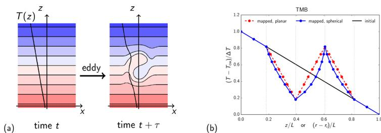
Figure 2: Schematic of an eddy turnover (a) and its 1-D representation due to the triplet map (b).
