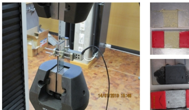
Fig. 2. Left: Short-term test set up Right: Failure modes of AC (above) and EP (below)
