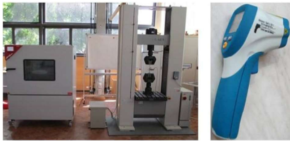
Fig. 2. Test equipment: left: the climate chamber close to the testing machine; right: the laser thermometer used for measuring the temperature at the surface of the specimen
