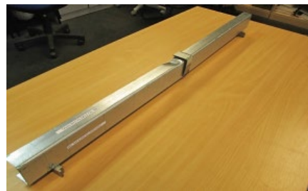
Fig. 3. Deformation of non-strengthened girder
