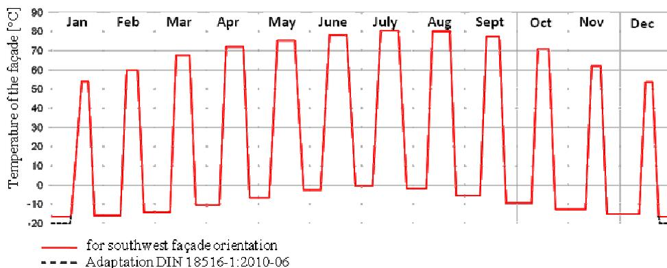
**Fig. 3.** Statistically determined temperature load cycle (Germany)
