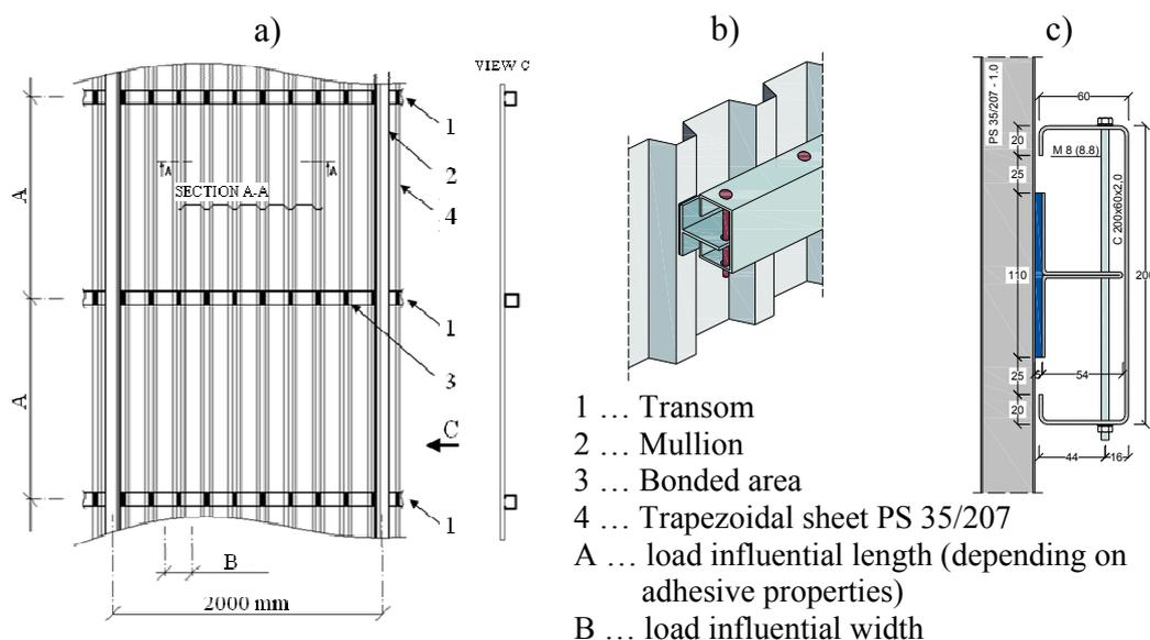
**Fig. 1.** Façade with adhesively bonded connections: a) technical view; b) schematic figure; c) cross section normal to the longitudinal axis
