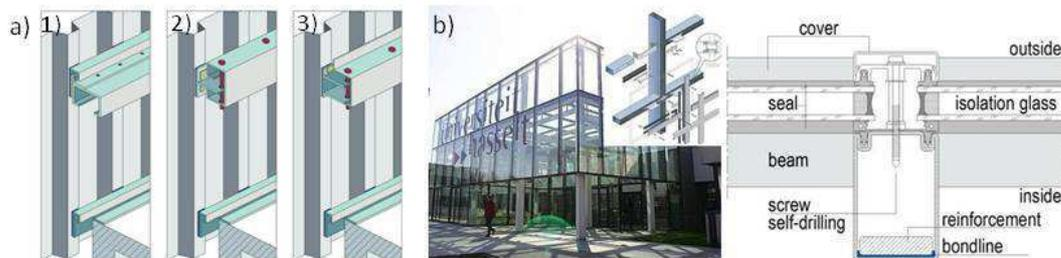
*Fig. 2.* a) Structures for bonded facade connections with different shape of connection profile 1) L-profile, 2) T-profile, 3) Pi-Profile; b) post and beam facade with bonded facade reinforcement [11]
