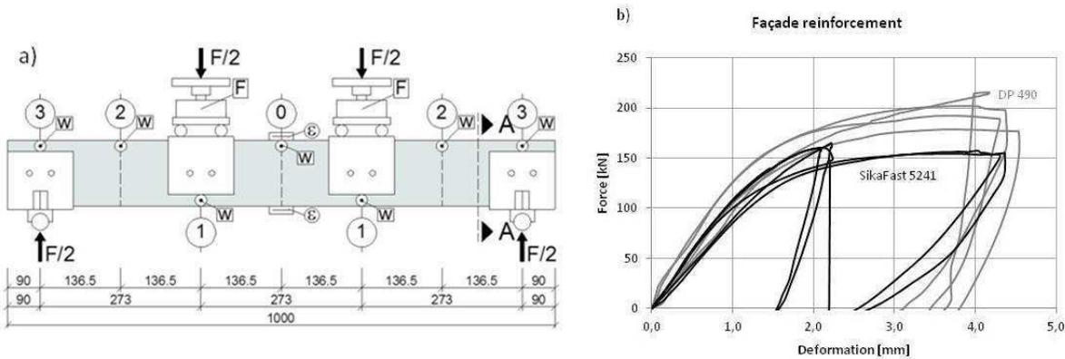
Fig. 5. a) Test setup; b) Test results
