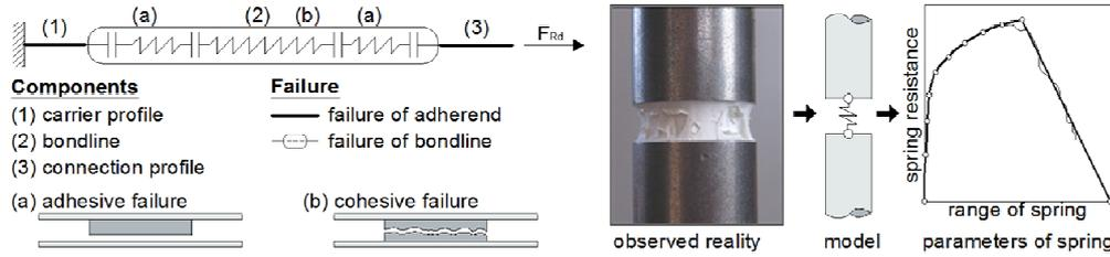
Fig. 6. Component-spring model
