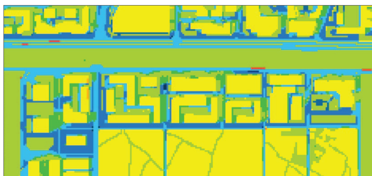
Fig. II-B.6: Reduction of surface temperatures when changing HCMC's conventional paving materials (cement and non-porous asphalt) to cool paving materials (porous asphalt and light coloured permeable bricks). Map is simulated by ENVI-met 04 under the climatic conditions of HCMC (Huynh & Eckert).
