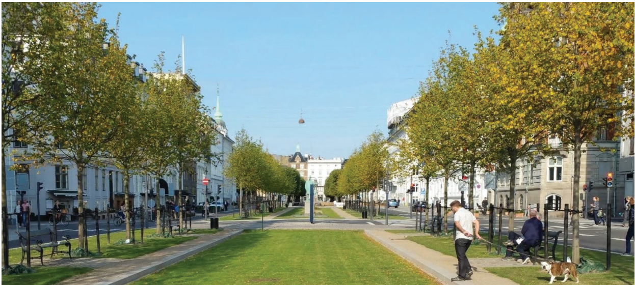
Fig. 2.17. Example of rain retention and seepage by creating a retention area in a street profile in Copenhagen (Denmark) [Source: Department of Urban Technical Infrastructure, BTU Cottbus Senftenberg]
