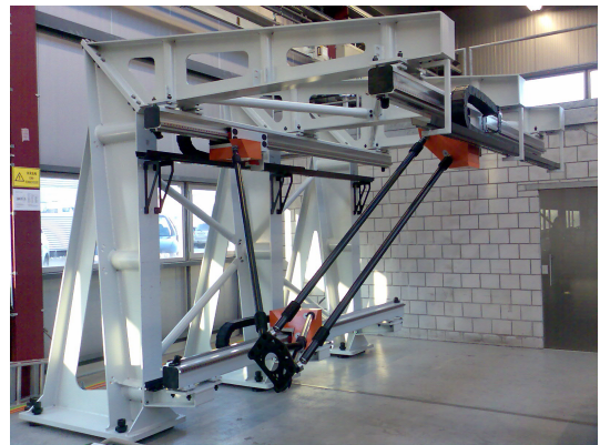
Figure 1: Full size Gantry-Tau prototype developed within the SMERobot TM project. The carts (red) are controlled in a coordinated way along the three rails to move the tool/end-plate along a desired trajectory.
