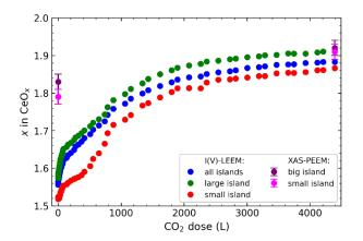
Figure 1: Reoxidation of cerium oxide islands by exposure to CO<sub>2</sub> at 550 °C obtained from *in situ* XAS-PEEM and I(V)-LEEM analyses.
