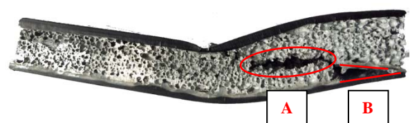
Fig.4: Failure mode A – Core failure Failure mode B – Delaminating interface
