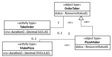
Figure 10: Making PizzaMaker an alternate resource pool for TakeOrder tasks.
