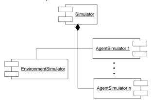
Figure 4: The AOR simulator architecture
