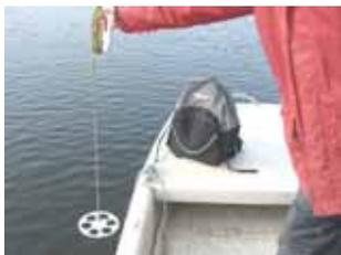
**Fig. 5:** Secchi disk used for determination of transparency depth.
