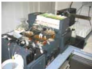
**Fig. 9:** Multichannel segmented flow analyzer
