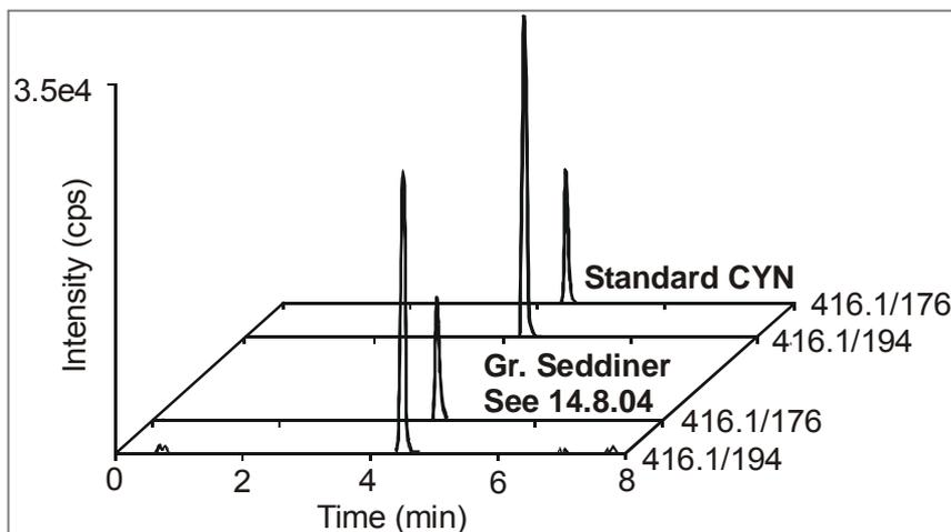
**Fig. 10:** Selected reaction monitoring (SRM) chromatogram for cylindrospermopsin standard and sample taken from Grosser Seddiner See on 14 Aug 2004 showing the characteristic transitions for cylindrospermopsin ( $m/z$  416.1/194 and 416.1/176).
