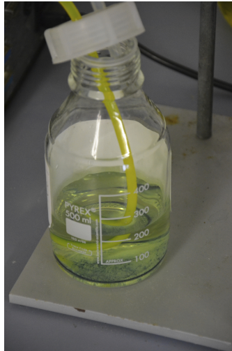
Picture 6: Bottle with the percolation solution with the visible blue precipitate in the bottom.
