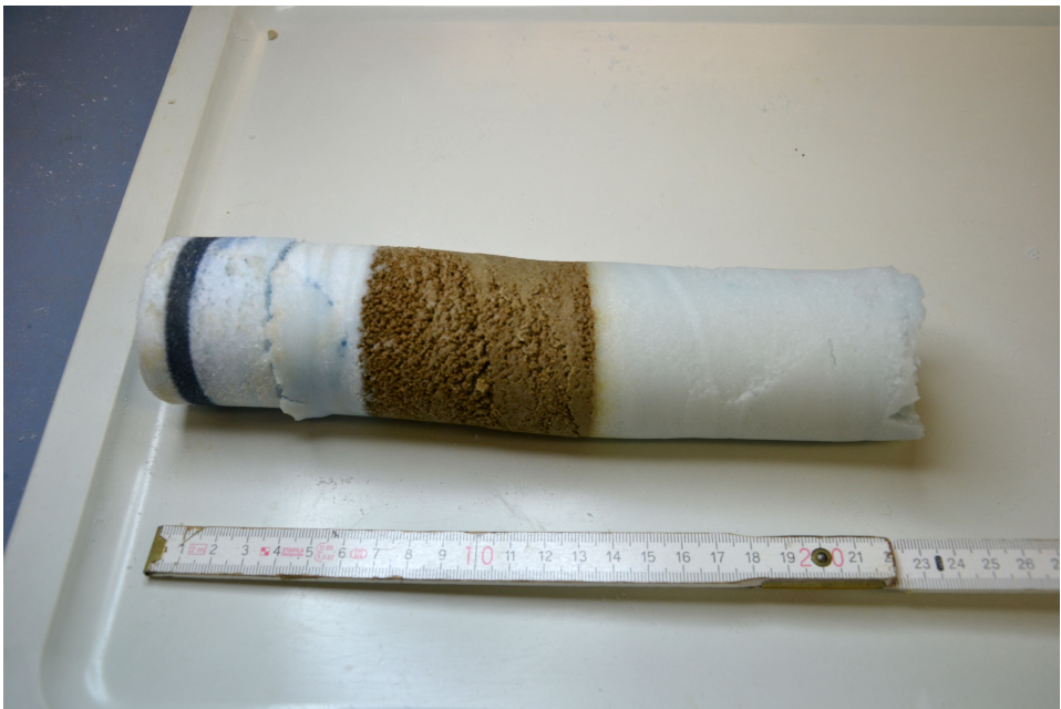
Picture 10: Disassembling of the column experiment and investigating the material.
