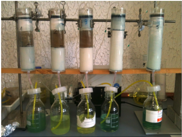
Picture 7: The 2 nd column experiment after 20 day of percolation.
