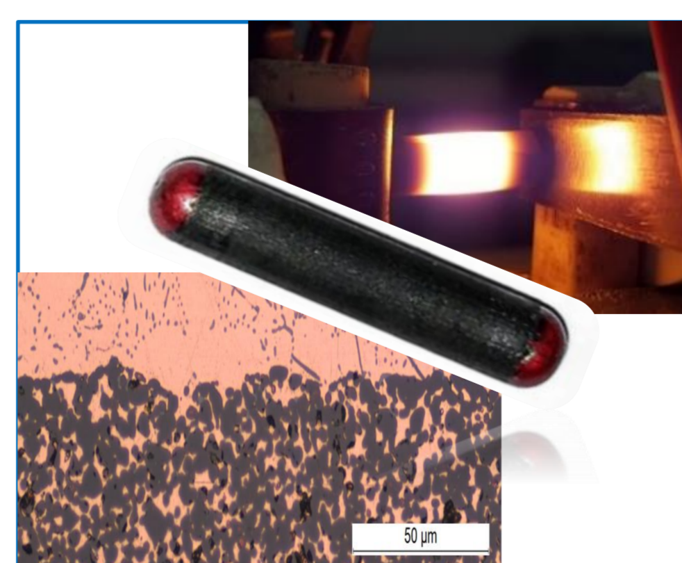
Multi-material design – conductive ceramics \text{LaCrO}_3 - Cu
