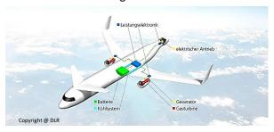
efficient electric motors to generate thrust using sustainable aviation fuels in fuel cells and gas turbines. However, there are many remaining challenges to be solved before the implementation of this technology and bring it into service.
