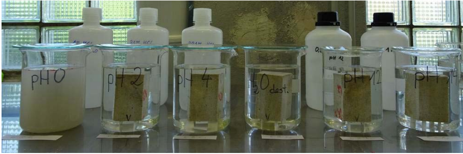
Fig. 10 —Experimental setup for the durability tests in a wide pH range (from 0 to 14)
