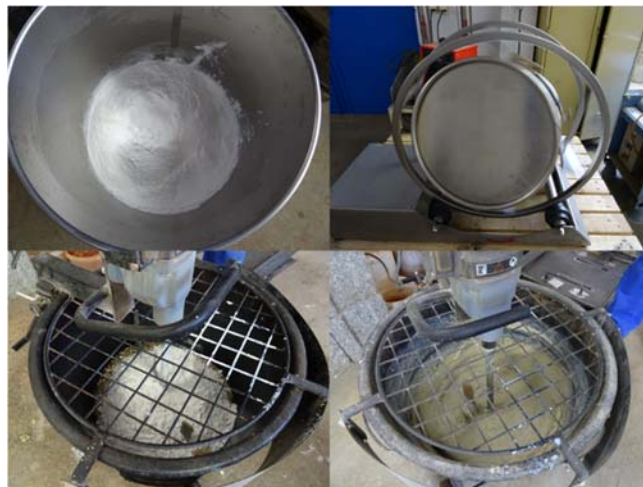
Fig. 5 –Manufacturing process of the specimens in the technical scale top left: container of the Rhoen wheel mixer, top right: Rhoen wheel mixer, bottom left: dry mixture sand +sodium aluminate, bottom right: mix procedure of all components
