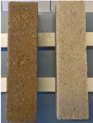
Fig. 11a —Mortar prisms stored in H_2SO_4 (pH 2) until 28 d (left cement, right ASN)
