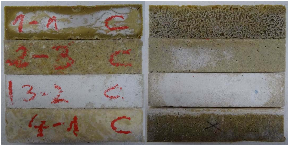
Fig. 6–Samples R1 to R4 from the manufacturing procedure after 28 d curing
