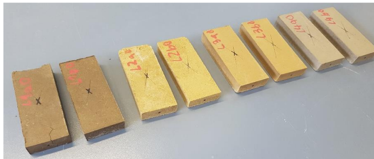
Fig. 3: Loam samples produced in the laboratory
