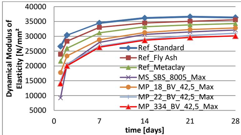
Fig. 3: Dynamical Modulus of Elasticity of mortar samples investigated
