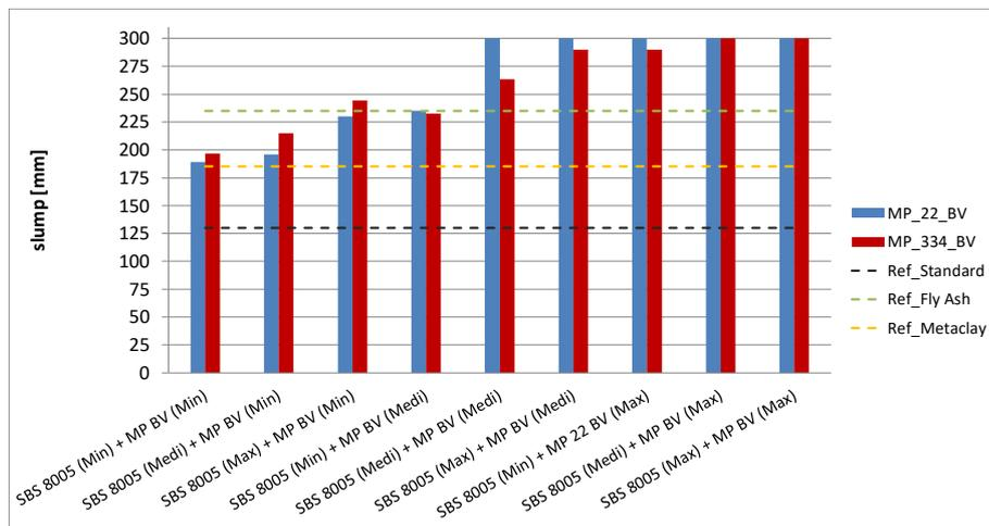
**Fig. 2:** Slump of samples produced with different superplasticizers in mixtures
