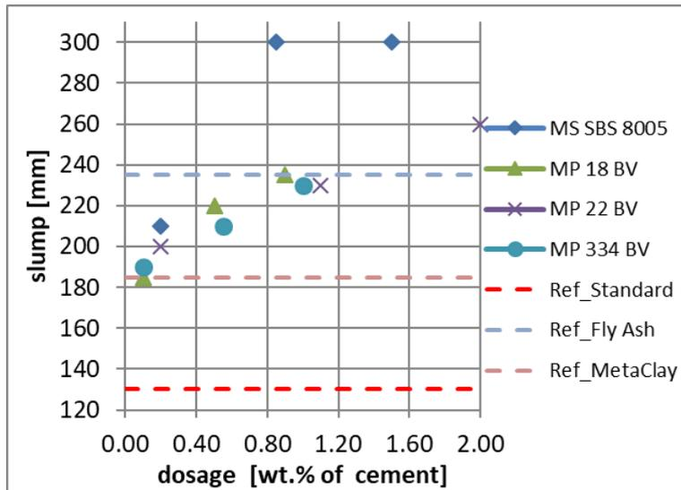
**Fig. 1:** Slump of samples produced with different superplasticizers
