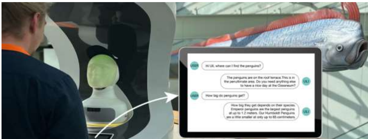
Figure 1 Interaction with the 41cm tall social robot head Furhat with an illuminated mask system at the OZEANEUM Stralsund. The robot head is mounted on a housing, which includes a display to show a manual and transcribed dialogue during interactions. Source: Ana Müller, Cologne Cobots Lab, CC-BY-NC SA 4.0
