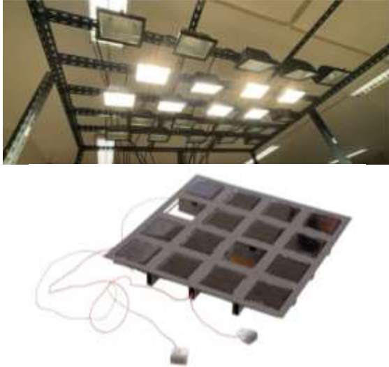
Figure 12: Greengrid prototype under solar simulator
