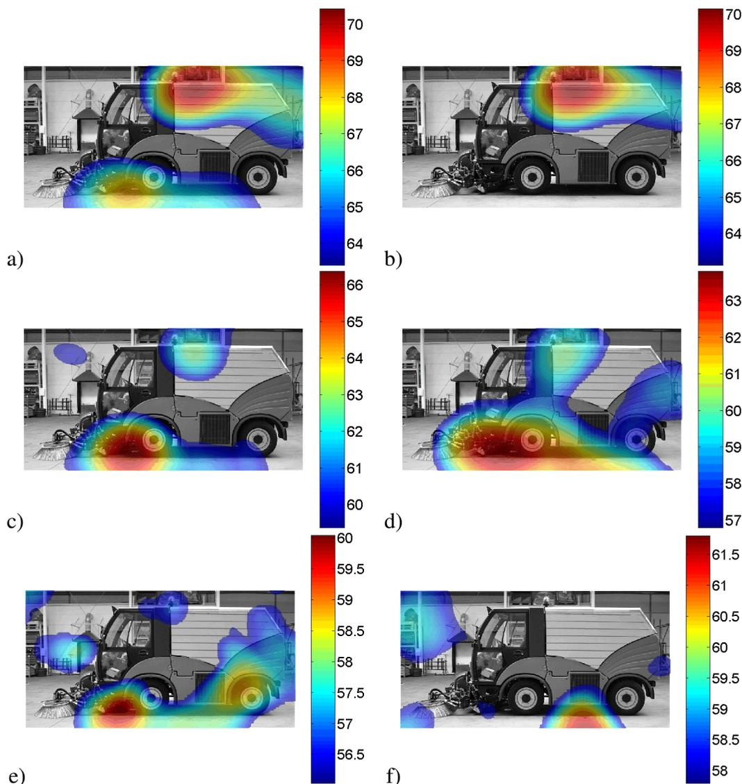
Figure 2: result maps from measurements on the cleaning vehicle (1.25 kHz third octave band): a) total and b)-f) first to fifth component corresponding to the blower, sucker(2x), brush and engine cooling
