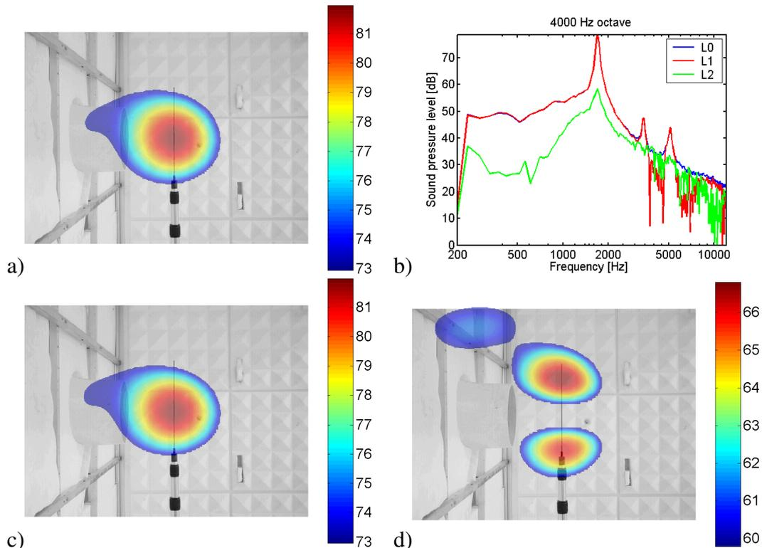
Figure 1: a) cylinder in Mach 0.11 open jet (nozzle at the left side of the picture), beamforming result map for the 2 kHz octave band, b) spectra of the overall result (L0) and the two first components (L1,L2) of the orthogonal beamforming result, c) first and d) second component of orthogonal beamforming result map for the 2 kHz octave band
