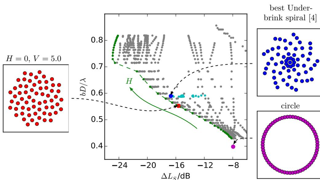
**Figure 6:** Beam width and sidelobe level for  $\frac{D}{\lambda} = 10$  and  $|\theta| < \frac{\pi}{4}$  for the proposed arrangements using (6) and (4) and different  $H$  and  $V$  (gray), for  $V = 5.0$  (green), for multi-armed logarithmic spirals after [4] (cyan) and a circle arrangement (magenta)
