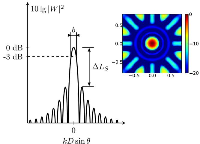
**Figure 1:** PSF Example with beam width  $b$  and minimum sidelobe level  $\Delta L_S$ .  $\theta$  gives the look direction from the array and  $k$  is the wave number. Inset shows a two-dimensional map of a similar PSF.
