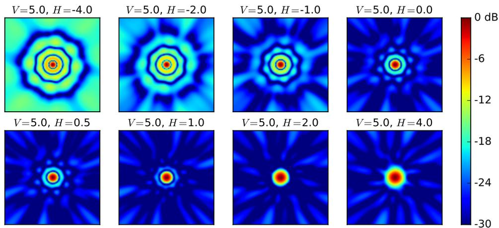
**Figure 5:** Point spread functions for the example arrangements shown in Fig. 4 for  $\frac{D}{\lambda} = 10$  and  $|\theta| < \frac{\pi}{4}$
