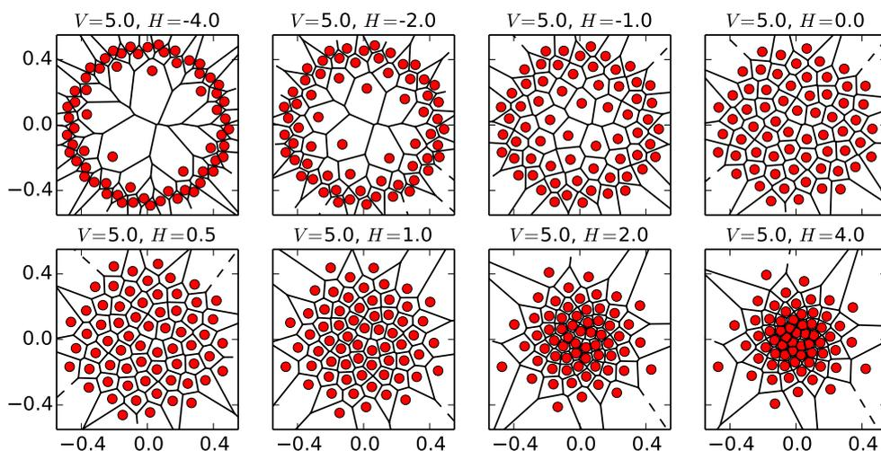
**Figure 4:** Examples for different arrangements with  $N = 64$  produced from (4) and (6) with Voronoi diagrams showing approximately the area per microphone
