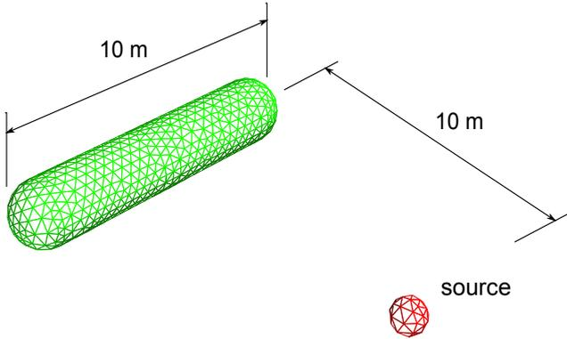
Figure 2: Example 1: scattering by a cylinder-shaped structure
