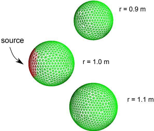
Figure 3: Example 2: three spheres with radiation from a sector on a sphere
