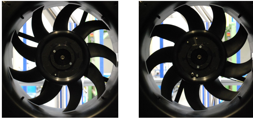
Figure 2. Fan with forward skewed blades (left) and backward skewed blades (right). Rotation is clockwise.
