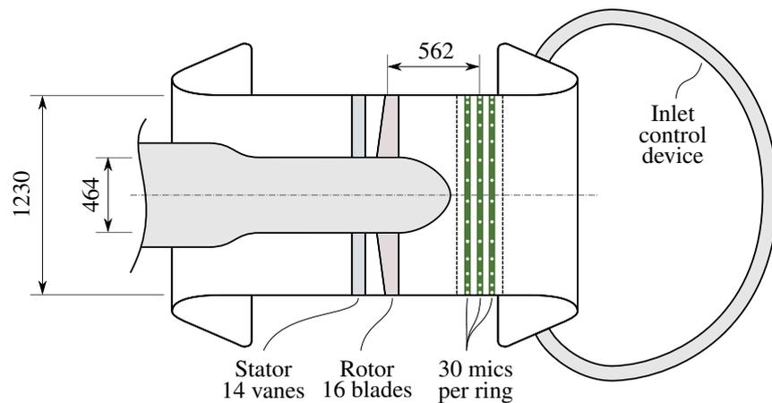
Figure 1: Schematic of the ANCF configuration used for the measurement, all values in mm.
