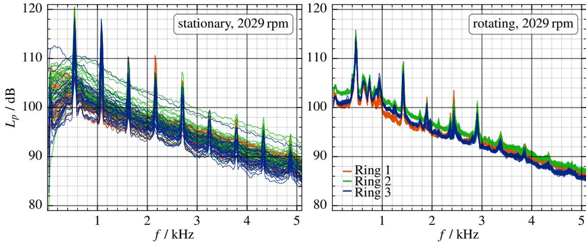
Figure 2: Microphone spectra in the stationary (left) and the virtual rotating (right) reference system. The rings are numbered against stream direction, i.e. Ring 1 is closest to the fan and Ring 3 is closest to the inlet.
