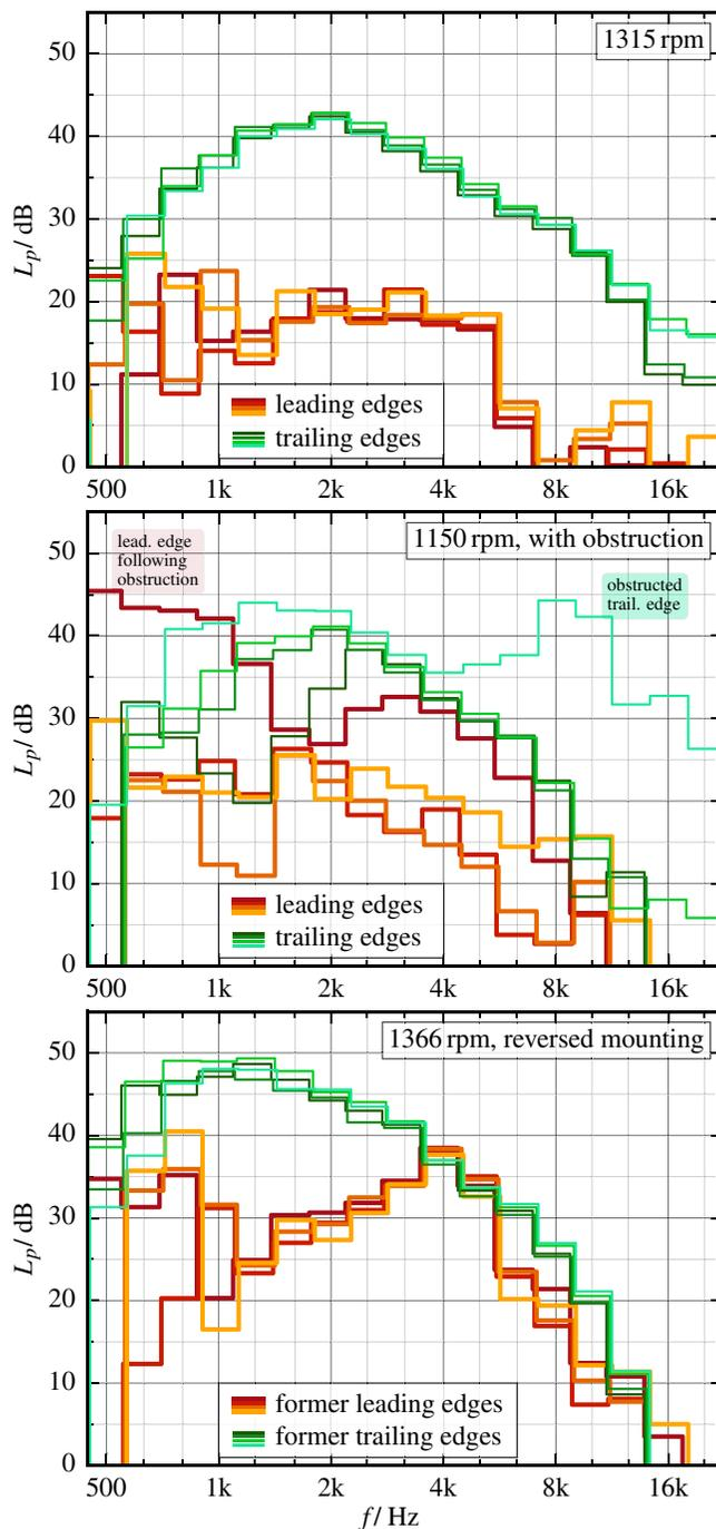
Fig. 5—Leading and trailing edge spectra (sound pressure level) for the fan at different operating cases. In the case of the backwards mounted fan, the slanted parts of the blades are facing the flow, i.e., the former trailing edge is in fact leading edge and vice versa.
