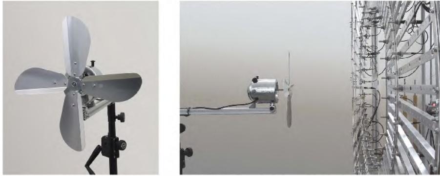
Fig. 1—Fan used for the measurements. Fan with microphone array (only the inner ring of microphones was used).
