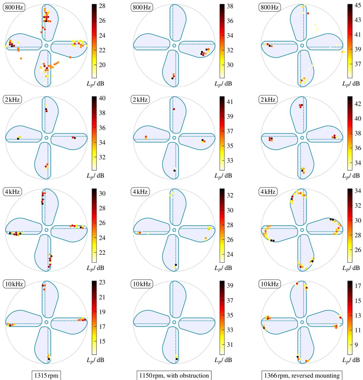
Fig. 3—CLEAN-SC sound maps for a clock-wise rotating fan using the virtual rotating array method. The results of three different measurement cases (columns) are evaluated at exemplary one-third octave bands (rows). Displayed are reconstructed sound pressure levels up to 10 dB below the respective band maximum level.
