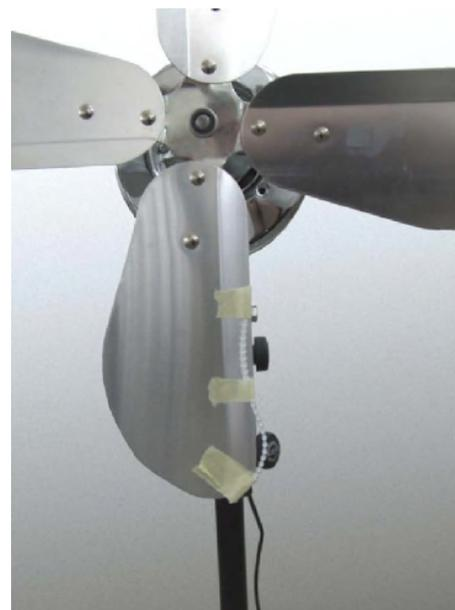
Fig. 2—Fan with applied flow obstruction (ball type cable tie) at the trailing edge of the blade at 6 o'clock.
