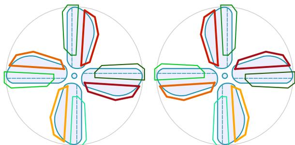
Fig. 4—Schematic of the fan with assigned integration sectors (left: normal mounting, right: reversed mounting). Shades of red: leading edges, shades of green: trailing edges.
