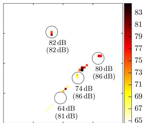
Figure 7. Example of a CLEAN-SC Map for  $He = 2$ , 1/3 octave. Circles indicate integration areas around the correct source positions.
