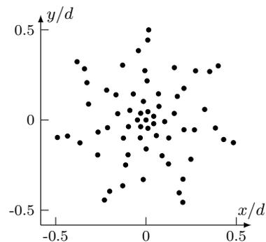
Figure 1. Array geometry with 64 microphones in one plane, aperture  $d$ .
