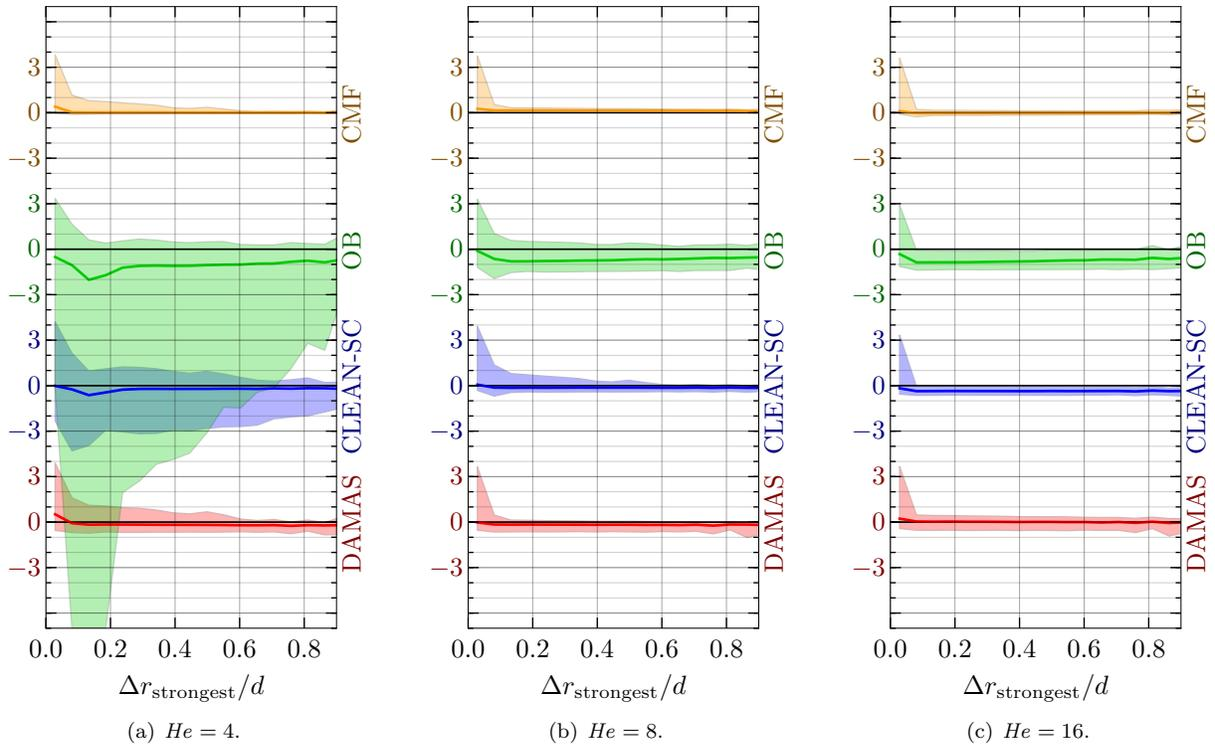
Figure 10. Relative level error  $\Delta L_{p, err}$  for different Helmholtz numbers, depending on the distance of the evaluated source to the strongest source.
