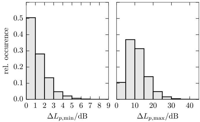
Figure 5. Scaled histogram of the minimum (left) and the maximum (right) level differences occurring between 4 source levels randomly drawn from the Rayleigh distribution.
