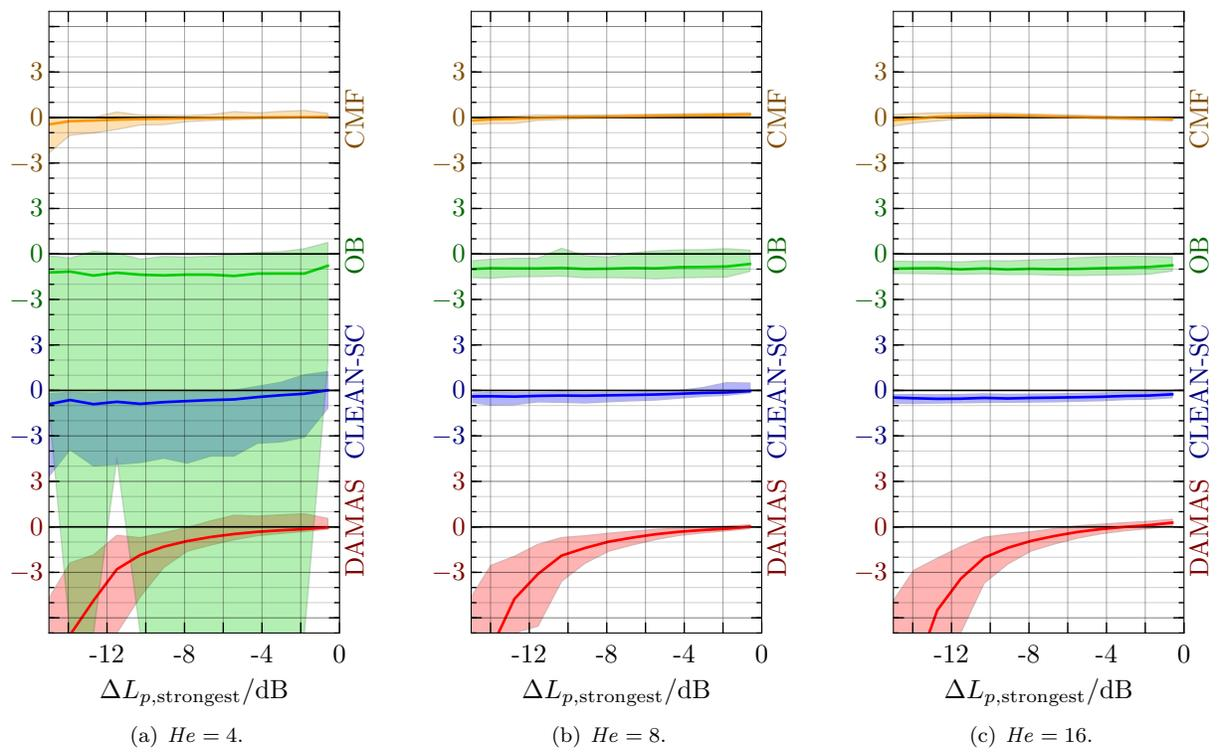
Figure 9. Relative level error  $\Delta L_{p, \text{err}}$  for different Helmholtz numbers, depending on level difference to the strongest source.
