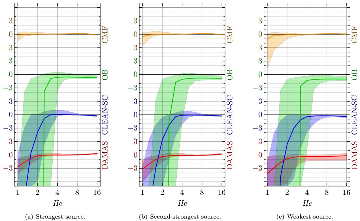
Figure 8. Relative level error  $\Delta L_{p, \text{err}}$  in dB for different sources, depending on the Helmholtz number.
