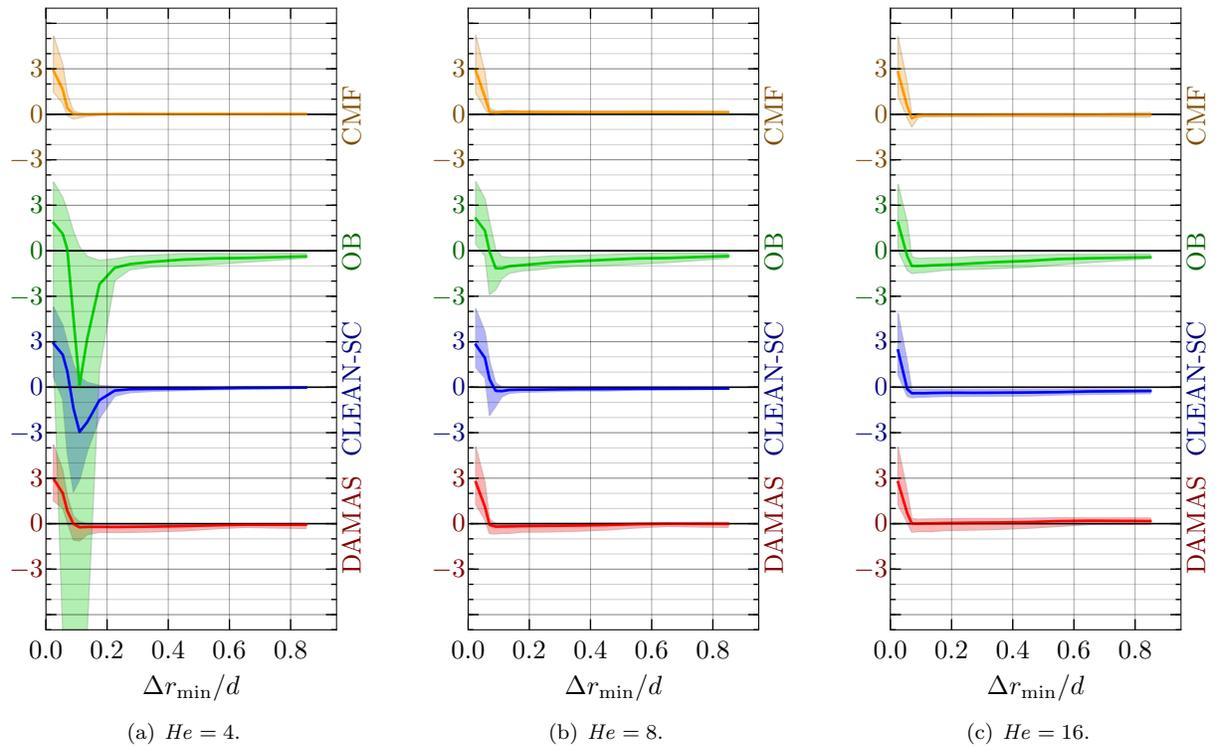
Figure 11. Relative level error  $\Delta L_{p, err}$  for different Helmholtz numbers, depending on the distance of the evaluated source to the nearest source.
