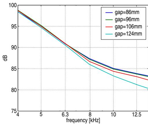
(a) fix rod diameter of 10 mm and varied gap
