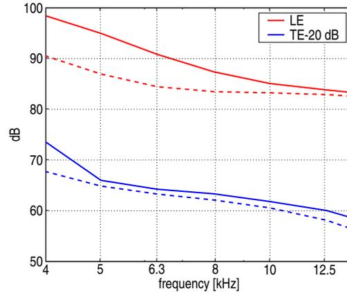
**Figure 4:** LE and the TE third octave spectra for the NACA 0012 (solid line) and the NACA 0018 (dashed line) airfoil for a configuration with a gap of 86 mm and a rod with 10 mm diameter.
