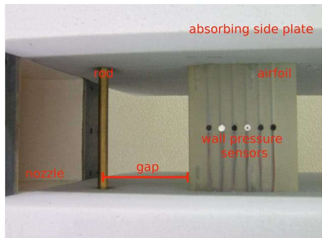
Figure 2: Rod-airfoil-configuration mounted between two absorbing side plates directly attached to the wind tunnel nozzle exit. The installed airfoil has flush integrated dynamic wall pressure sensors.
