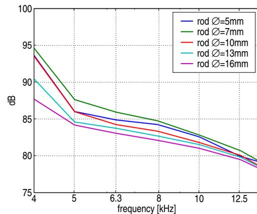
(b) fix gap of 86 mm and varied rod diameter
