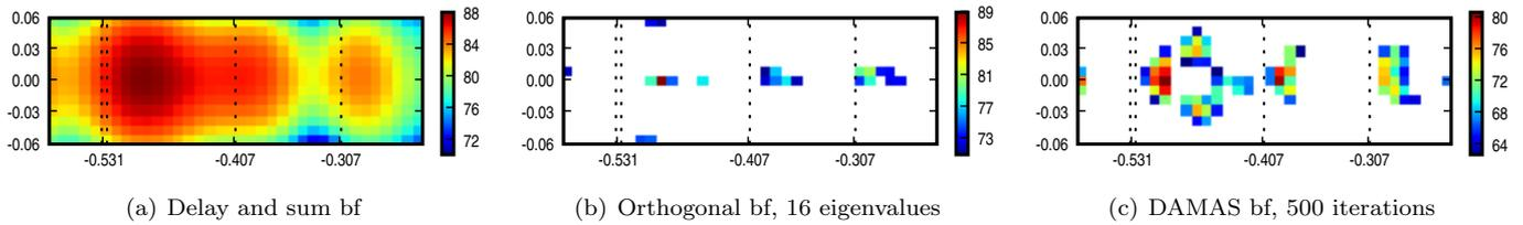
**Figure 3:** Comparison of the spatial resolution of different beamforming (bf) algorithms on a rod-airfoil-configuration. Shown are pictures for a flow speed of 72 m/s and the 5 kHz third octave band (flow from left to right).
