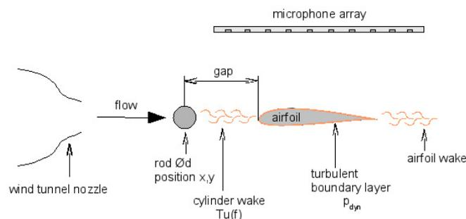
Figure 1: Schema of the experimental setup.
