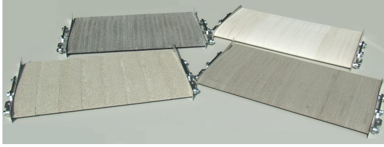
Figure 2. Photograph of the porous airfoils, from upper left to lower right: M-Pore Al 45 ppi, Porex, Reapor, Recemat)
