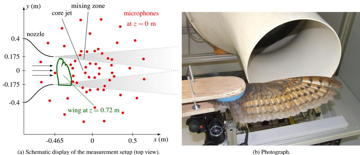
Figure 8 – Setup of the measurements on prepared wings in the aeroacoustic wind tunnel.
