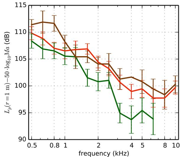
Figure 7 – Scaled third octave band sound pressure levels obtained from the flyover measurements presented in (16): ■ barn owl, ■ harris hawk, ■ common kestrel.
