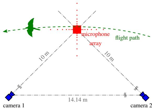
(a) Schematic of the measurement setup.
