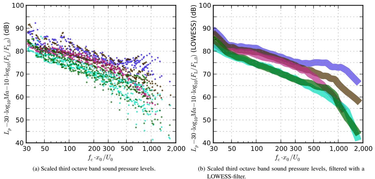
Figure 9 – Results from the wind tunnel measurements on prepared bird wings as presented in (30): ■ barn owl, ■ tawny owl, ■ common buzzard, ■ eurasian sparrowhawk, ■ pigeon.
