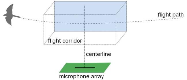
**Figure 1:** Measurement setup, the bird is gliding over the microphone array through a flight corridor
