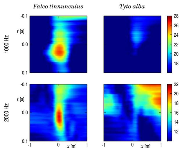
**Figure 4:** Preliminary results: octave band sound pressure level as a function of time (vertically) and position relative to the bird (horizontally), left: Common Kestrel, right: Barn Owl
