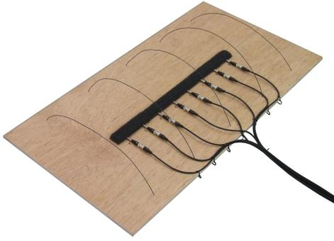
**Figure 2:** 8 channel microphone array, board with wire bows to apply a camouflage cover
