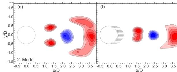
**Abbildung 4:** Comparison of 2nd POD mode of spanwise vorticity for reference cylinder (left) and hair flaps (right)
