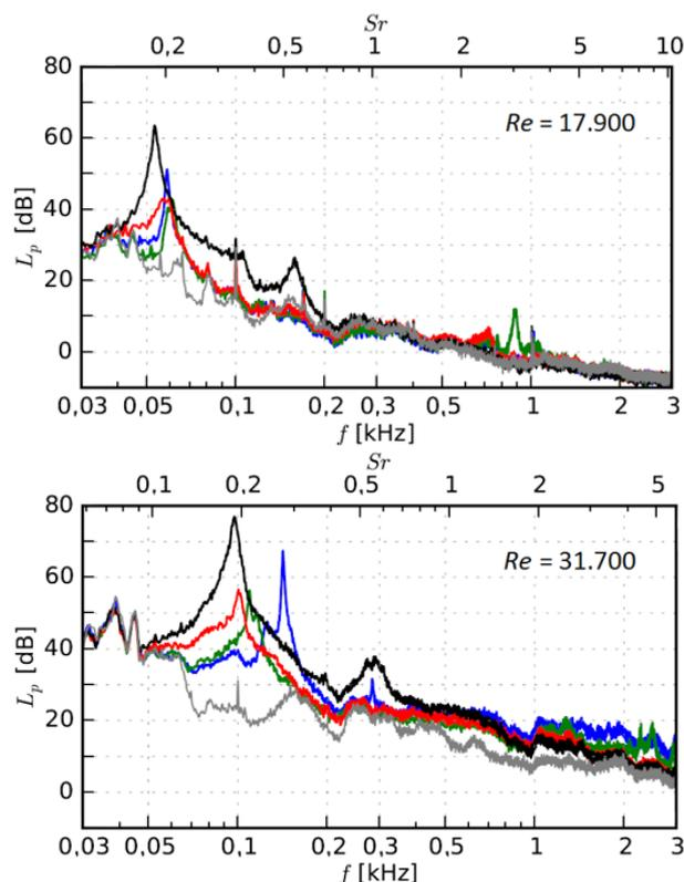
Abbildung 6: Sound spectrum for different Reynolds-numbers (black line: reference cylinder; blue line: hairy flaps)
