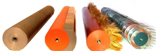
**Abbildung 1:** Models of the cylindrical test objects investigated within the anechoic wind-tunnel
