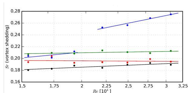
**Abbildung 5:** Plot of Strouhal over Reynolds-number for the reference cylinder (black line) and the hairy flaps (blue line)
