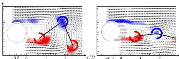
**Abbildung 3:** Comparison of wake flow pattern for reference cylinder (left) and hair flaps (right)
