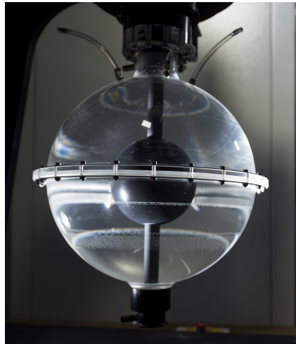
Figure 2: Experimental setup. Radius of the inner and outer sphere is 40mm and 120mm. Both spheres can rotate independently. Libration can be superposed on the rotation of both spheres.
