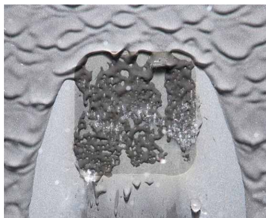
Figure 1: The flow of a water film moving under the action of gas in a 1.5 mm high channel with a heater of 1x1 cm 2 . Reynolds number of liquid Re_l = 14 , superficial gas velocity U_{sg} = 34 m/s, heat flux q = 240 W/cm 2 , temperature of the heater surface T_w = 126^\circ\text{C} . The flow is directed from top to bottom.
