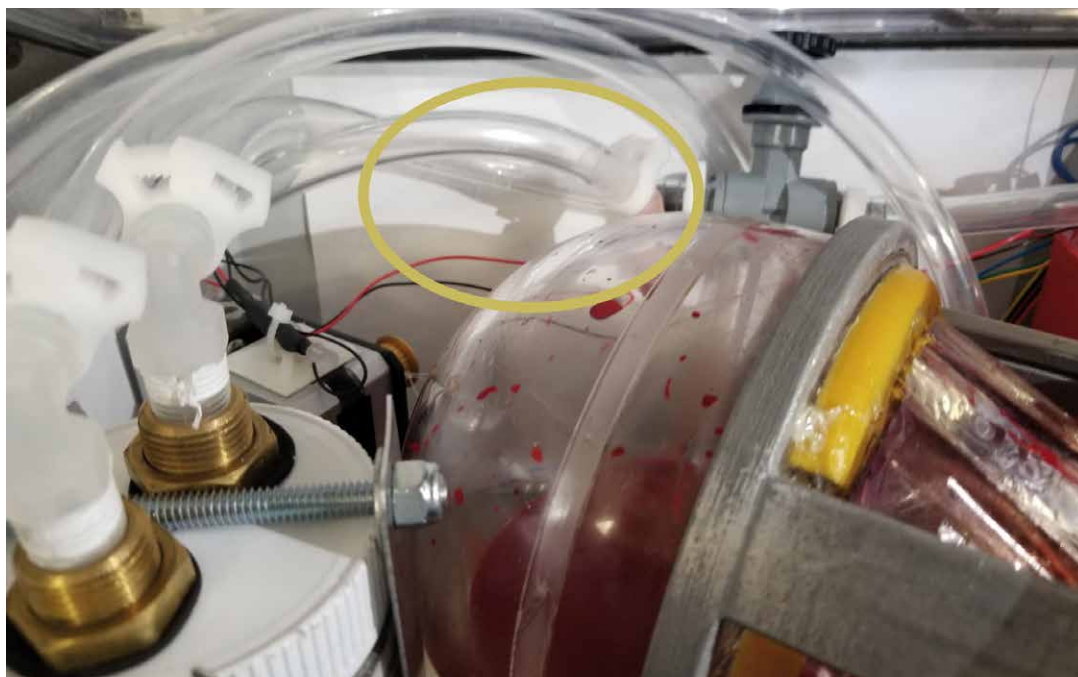
Figure 4. Post-flight condition of the third test. The gold ellipse highlights the air vent from the separator which is clean of all blood.
