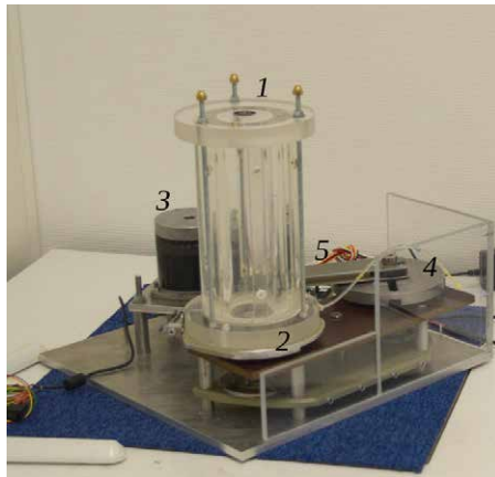
Figure 1: Experimental setup: 1 – container, 2 – rocking platform, 3 – motor, 4 – crank, 5 – rod.
