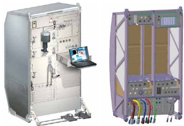
Figure 2: Left: Fluid Science Laboratory (FSL) Right: European Drawer Rack 2 (EDR2)
