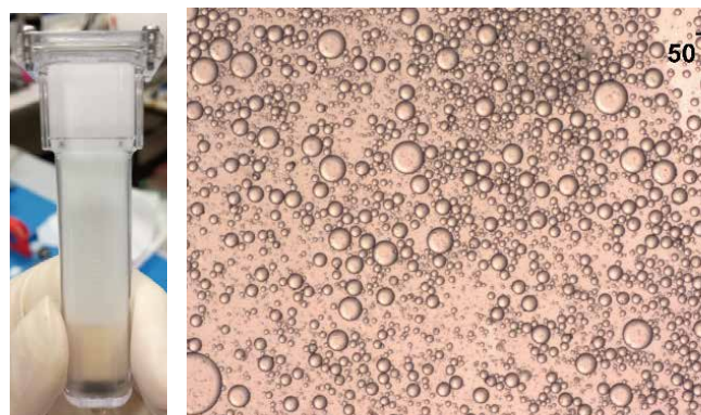
Fig.1 left, the cell employed for emulsification, right, micrograph of the obtained emulsion
