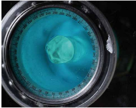
Figure 2: Photograph of the two-liquid system at rotation taken through the front flange at some angle to the rotation axis.
