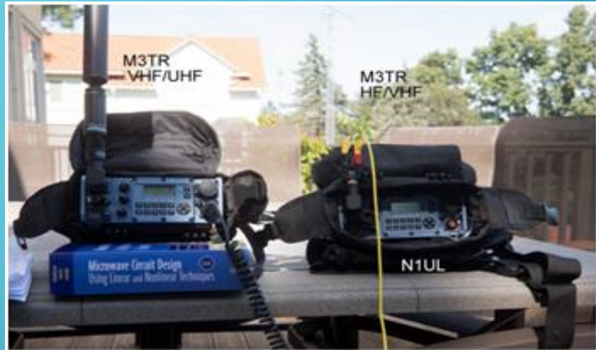
VHF/UHF (left) and HF/VHF (right) manpacks. The UHF/VHF manpack shown uses a thick vertical pole antenna, and the HF manpack uses a 5 m dipole (the yellow wire).
