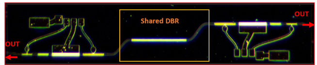
▲ Fig. 6 Shared DBR-based multimode semiconductor laser with symmetric multi-section multimode lasers on the left and right of a shared DBR. Chip dimensions = 4.6 mm x 1.2 mm.
