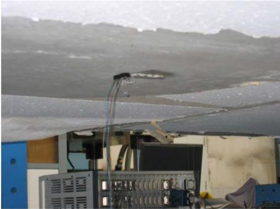
Fig. 6.8: Strain gauges in the tension zone
