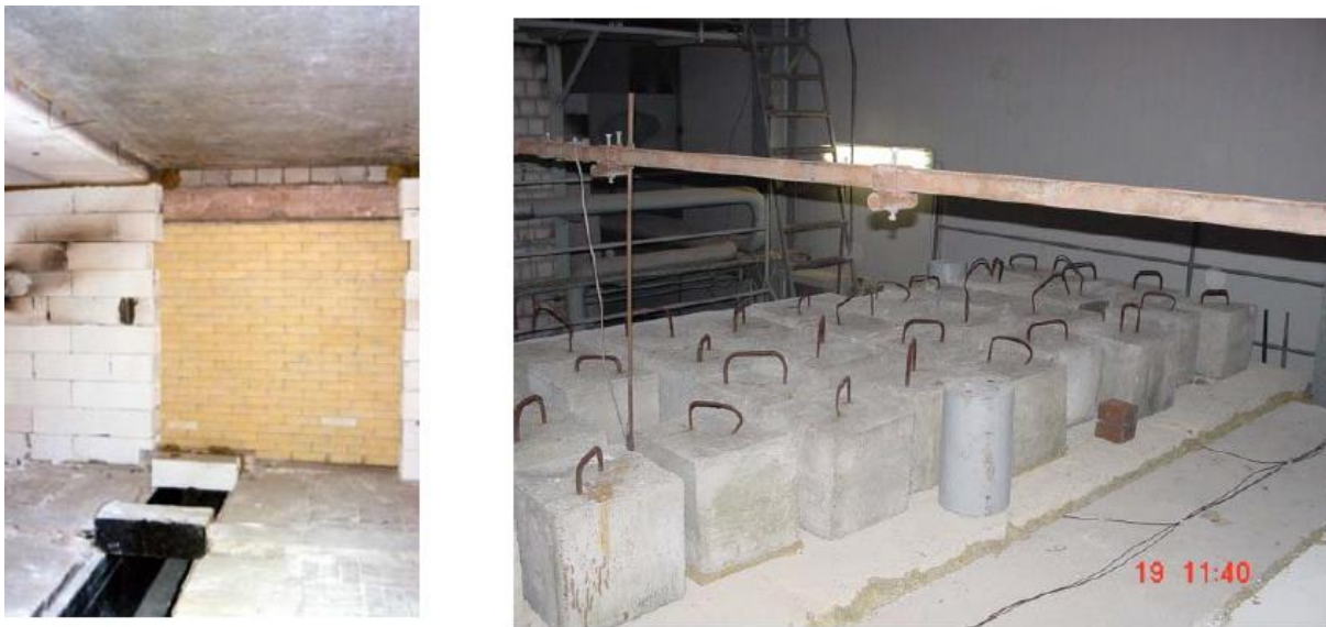
Fig. 6.21: Fire test room (left) and simulation load (right)
