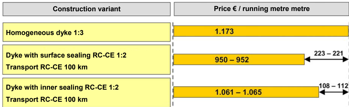
Fig. 7.13: Comparison of construction costs of different dyke variants with details of cost-saving potential
